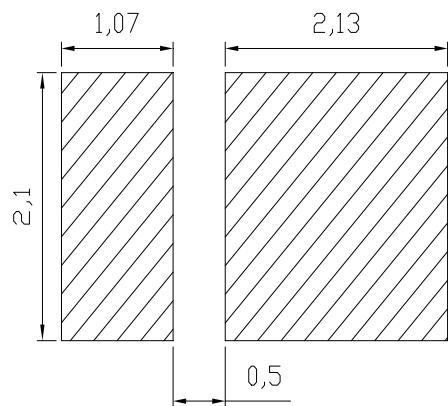
For reflow soldering
