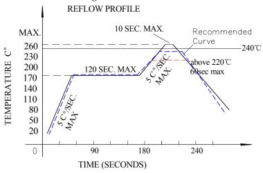
Reflow soldering curve
