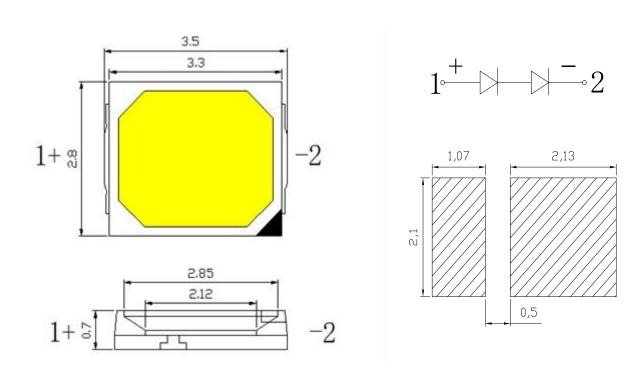
For reflow soldering
